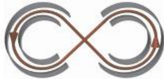
(f) Multiple-Turn TOF-MS (open path)
