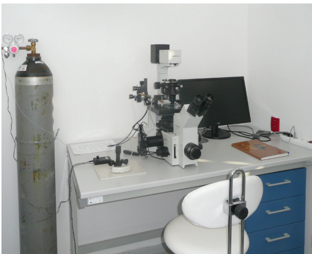
Microscope Olympus IX70 with a complete microinjection system for preparation of transgenic organisms. © Marta Kostrouchová
