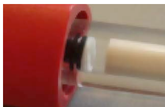
Fig A4.2. The maximum pressure over the packed bed is the maximum pressure the packed bed of chromatography medium can withstand without gap formation. This is not a fixed value.
