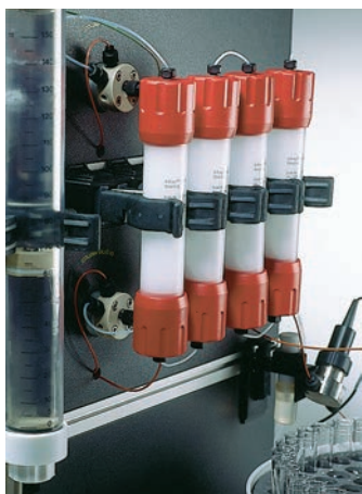
Fig 5.9. Four HiPrep 26/10 Desalting columns connected in series.
