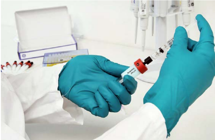
Fig 5.8. HiTrap Desalting column operated by syringe.
