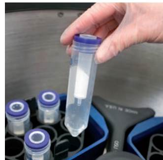
Fig 5.14. Spin adapters enable the use of PD-10 Desalting column, as well as PD MidiTrap G-25 and PD MiniTrap G-25 columns in a standard centrifuge.
