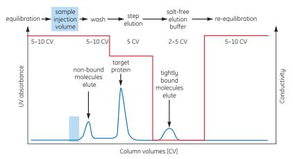
Fig 16. Typical HIC separation using step elution.
