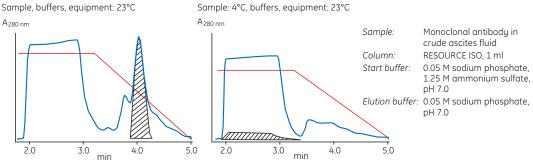
Fig 24. Influence of temperature on a HIC separation.
