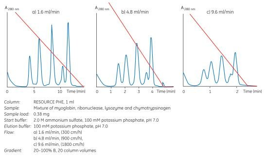
Fig 28. Influence of increasing flow rate on resolution when separating a model protein mixture on RESOURCE PHE.
