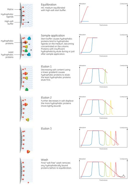
Fig 5. Steps in a HIC separation.
