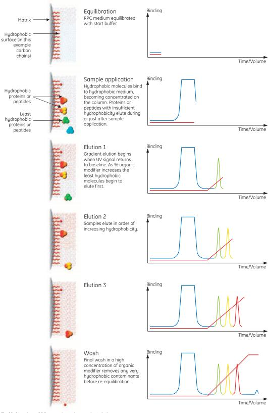
Fig 62. Steps in an RPC separation using gradient elution.
