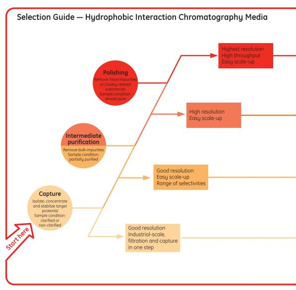
Fig 18. A typical purification strategy has three phases: Capture, Intermediate Purification and Polishing (CIPP). Each phase has a specific objective, dependent largely on the properties of the starting material. Select the appropriate HIC medium according to the objective of the purification step and the condition of the starting material.
