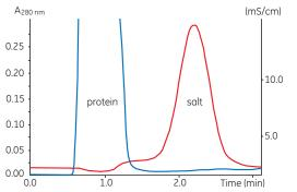
Fig 87. Buffer exchange of mouse plasma (10 ml) on HiPrep 26/10 Desalting.
