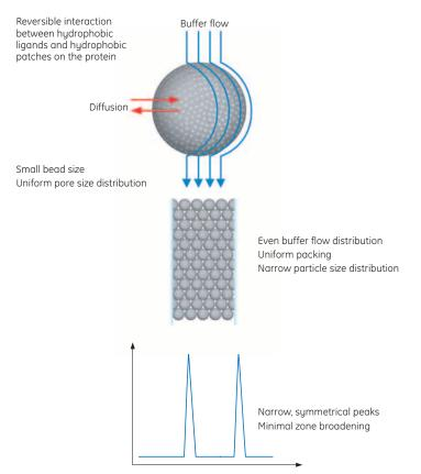
Fig 8. Factors that affect column efficiency.
