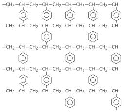
Fig 68. Partial structure of a polystyrene-based RPC medium.
