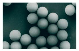
Fig 12. Electron micrograph of SOURCE showing spherical, monodispersed particles.
