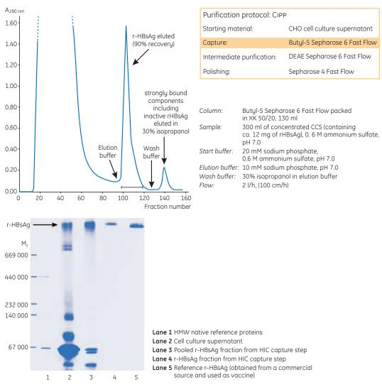
**Fig 46.** Large-scale purification of rHBsAg. Over 90% of impurities are removed by the HIC capture step (lane 3). Electrophoretic analysis (Gradient PAGE 4–30% under non-denaturing conditions) shows how purity increases after each chromatography step. r-HBsAg is a particle of 22 nm hence the band is seen at the top of the gel.
