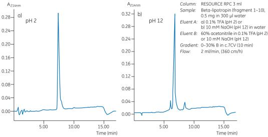
Fig 82. Purification at high pH.
