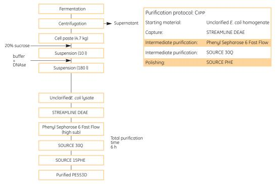
Fig 56. Four-step purification process.
