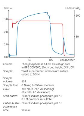
Fig 54. Development and scale-up of the capture step.
