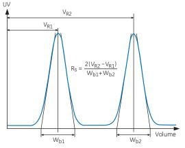
Fig 63. Determination of the resolution (R<sub>s</sub>) between two peaks.
