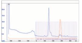
Column: Phenyl Sepharose 6 Fast Flow (high sub) packed in XK 16/10, 20 ml Sample volume: 50 ml, pooled from SP Sepharose Fast Flow Start buffer: 1.0 M ammonium sulfate, 30 mM phosphate, pH 6.0 Elution buffer: 30 mM phosphate, pH 6.0 150 cm/h, (5 ml/min) Flow: Gradient: 0-100% elution buffer in 20 CV System: ÄKTAexplorer
