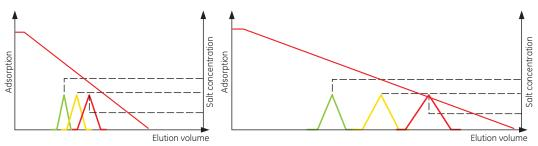
Fig 26. Schematic chromatograms showing the effect of decreasing gradient slope.
