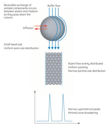
Fig 65. Factors that affect column efficiency.
