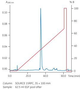
Sample: 62.5 ml EGF pool after Q Sepharose High Performance Load: 0.1 mg/ml media. 10 mg total load Eluent A: 0.05% TFA, 5% acetonitrile Eluent B: 0.05% TFA, 80% acetonitrile Gradient: 0–100% B in 40 CV Flow: 50 ml/min, (300 cm/h)
