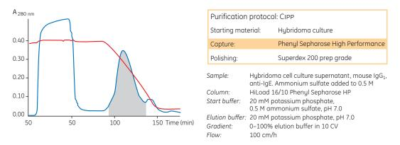
Fig 40. Concentration and purification of a monoclonal antibody from hybridoma cell culture.
