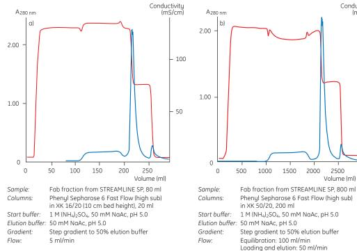
Fig 47. Intermediate purification and scale-up of a Fab fragment on Phenyl Sepharose 6 Fast Flow (high sub).
