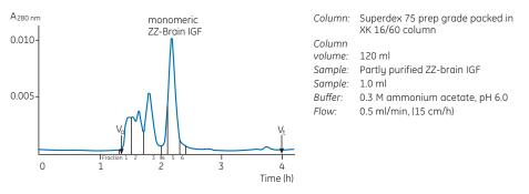
Fig 58. Final polishing step: separation of monomers, dimers and multimers on Superdex 75 prep grade.
