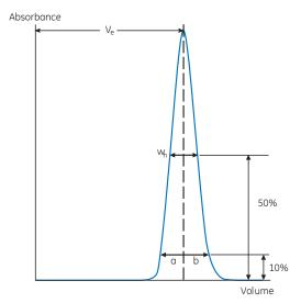
Fig 89. Measurement of efficiency.
