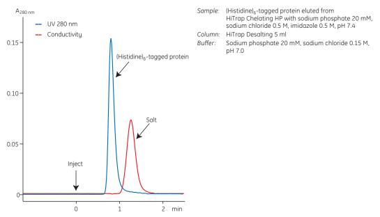
Fig 88. Desalting of a (Histidine),-tagged fusion protein on ÄKTAprime Plus.
