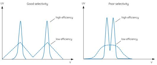
Fig 9. Effect of selectivity and efficiency on resolution.
