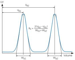
Fig 6. Determination of the resolution (R<sub>s</sub>) between two peaks.
