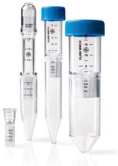
Fig 11.13. Vivaspin sample concentrators provide up to 30-fold concentration of the sample with recovery of the target molecule typically exceeding 95%.
