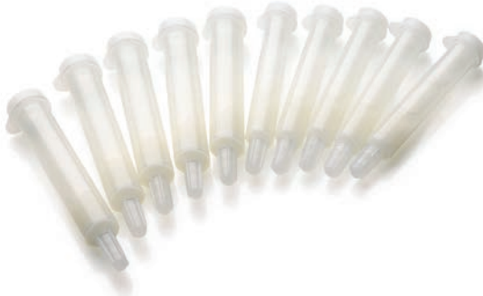
Fig 11.9. PD MidiTrap G-10 (left) and PD MiniTrap G-10 (right) columns are prepacked with Sephadex G-10.
